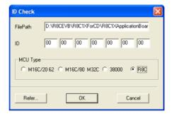
Select the file to be downloaded into the flash. Enter the ID as 0 initially as shown and select 'R8C option' in the MCU type. A screen appears as shown below.
